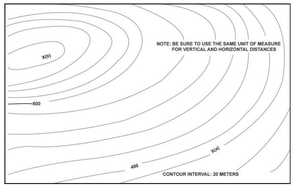
Figure 9-10. Contour lines around a slope
