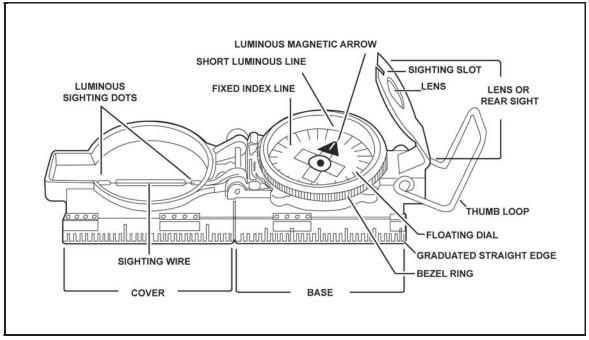
Figure 8-1. Lensatic compass
