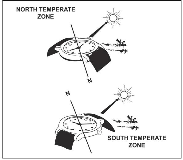
Figure 8-8. Determining direction using a watch
