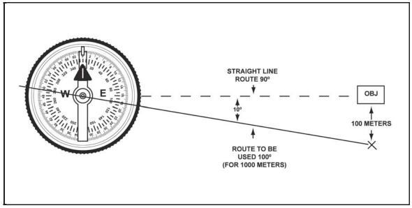
Figure 8-6. Deliberate offset to the objective
