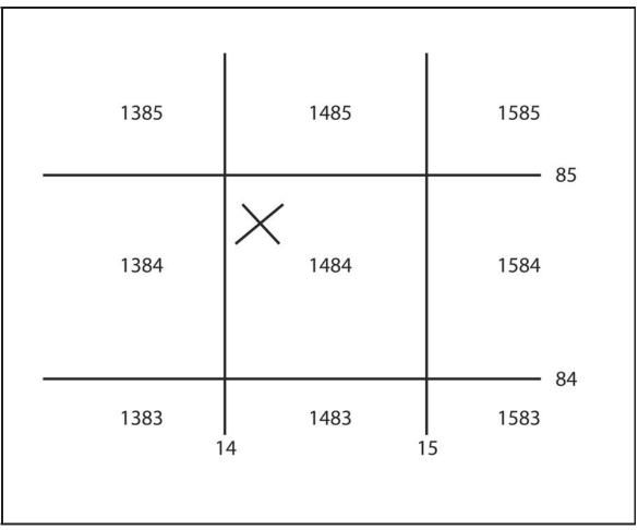
Figure 4-17. Determining grids without coordinate point
