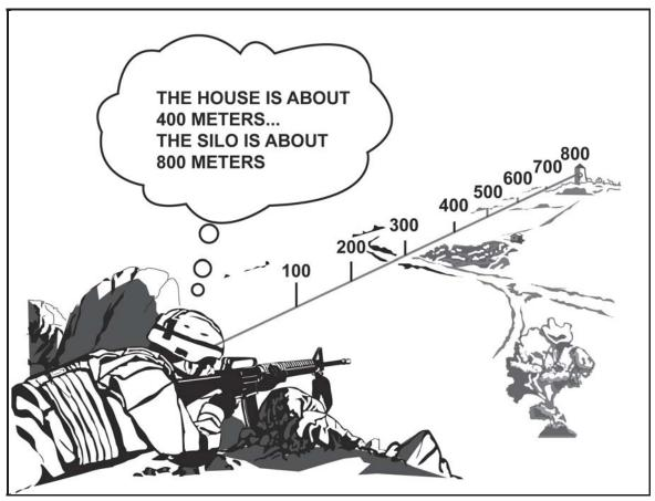
Figure 5-9. Using the 100-meter unit-of-measure method
