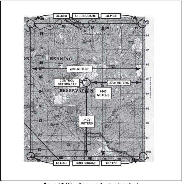
Figure 4-7. Using the proportional parts method
