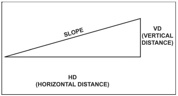
Figure 9-9. Slope diagram
