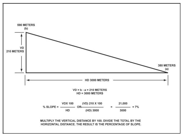
Figure 9-12. Percentage of slope in meters
