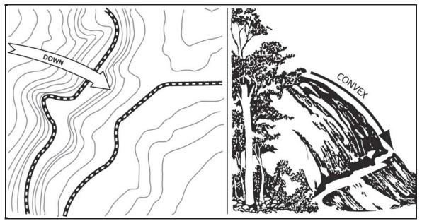
Figure 9-8. Convex slope
