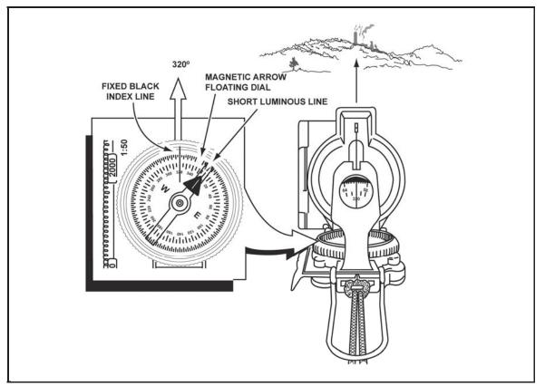
Figure 8-4. Compass preset at 320 degrees
