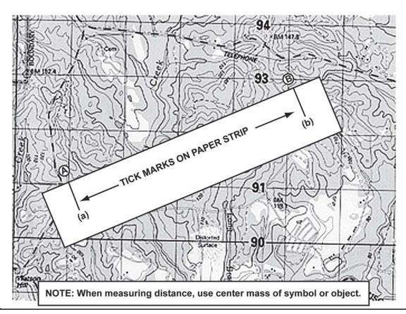
Figure 5-3. Transferring map distance to a paper strip
