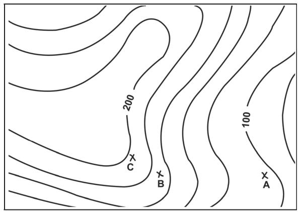
Figure 9-3. Points between contour lines
