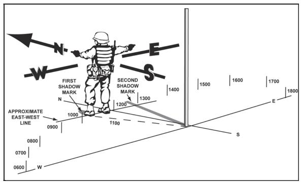
Figure 8-7. Determining directions shadow
