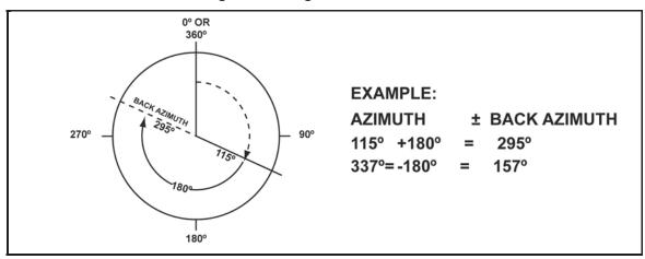
Figure 6-3. Back azimuth calculation with azimuth less than 180 degrees
