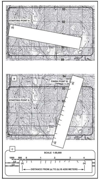
Figure 5-5. Measuring a curved line
