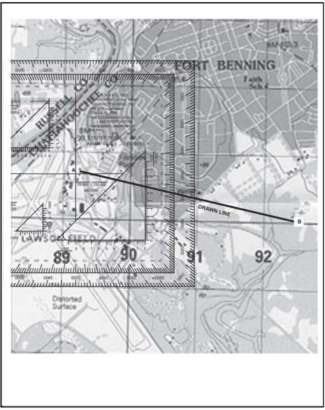
Figure 6-4. Measuring an azimuth
