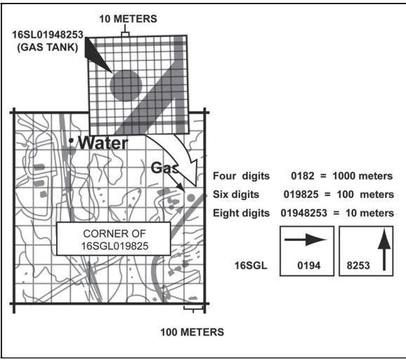
• **Precision.** The precision of a point's location is shown by the number of digits in the coordinates; the more digits, the more precise the location. (See Figure 4-22, insert.)
