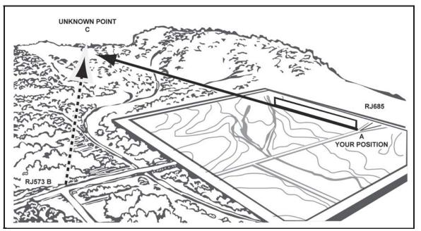
Figure 6-10. Intersection, using a straightedge
