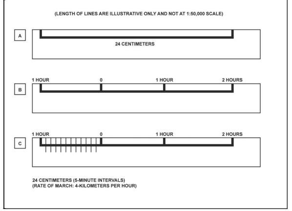
Figure 5-8. Constructing a time-distance scale
