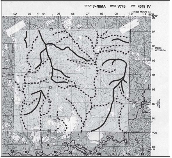
Figure 9-26. Ridgelining and streamlining
