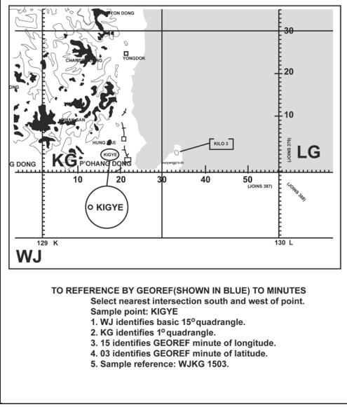
Figure 4-24. Sample reference using GEOREF
