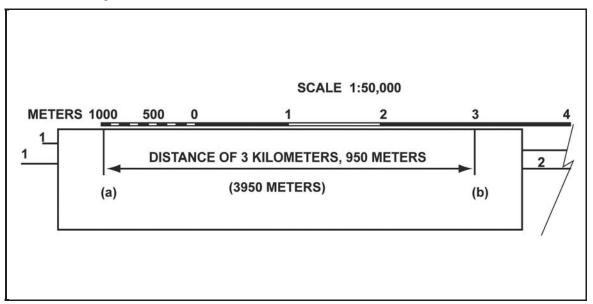
Figure 5-4. Measuring straight-line map distance
