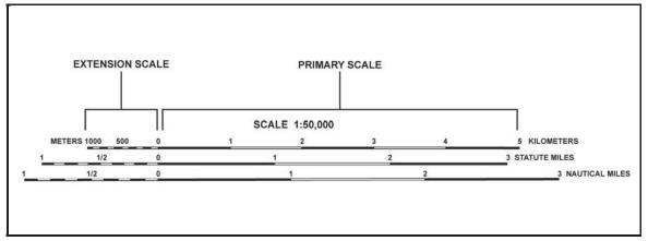
Figure 5-2. Using a graphic (bar) scale
