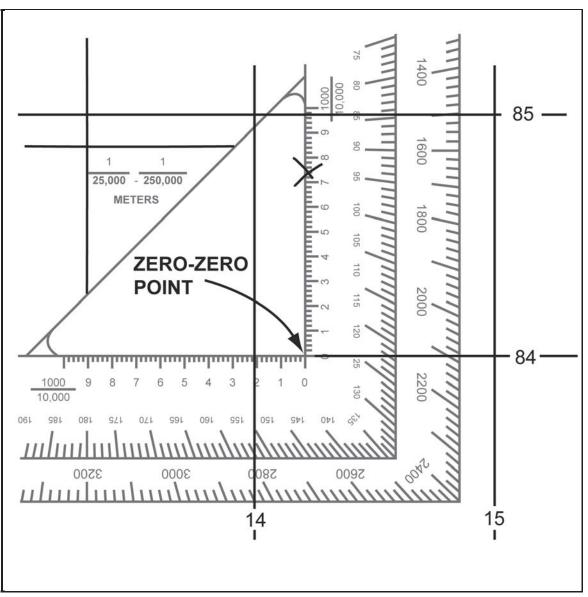
Figure 4-18. Placing a coordinate scale on a grid
