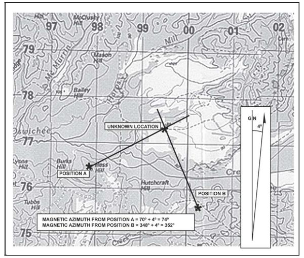
Figure 6-9. Intersection, using map and compass
