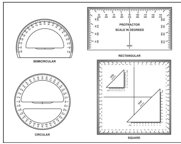
Figure 6-5. Types of protractors
