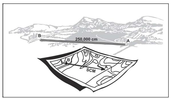
Figure 5-1. Converting map distance to ground distance
