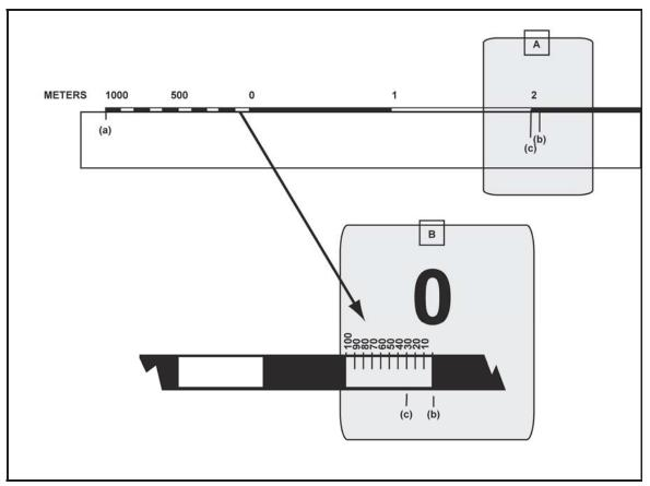
Figure 5-7. Reading the extension scale
