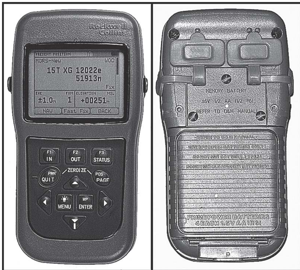
Figure I-1. Defense advanced GPS receiver (DAGR)
